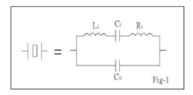
There are two zero-phase frequencies associated with this simple circuit, one is at series resonance fs, another at antiresonance fa. When used in an oscillator, crystal units will operate at any frequency within the broken lines of Fig-2 as determined by the phase of the maintaining circuit.
