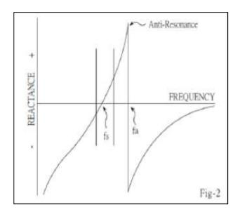
By changing of this reactive condition, the crystal frequency may be trimmed in a limited extent. The degree to which this frequency may be varied (frequency pulling) is inversely proportional to the capacitance ratio  $r(C_0 / C_1)$ .
