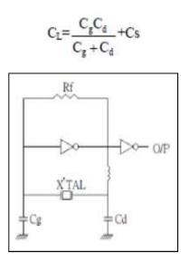
Cs: is the stray capacitance of the circuit typically the Cs value around 4\_8 PF.
