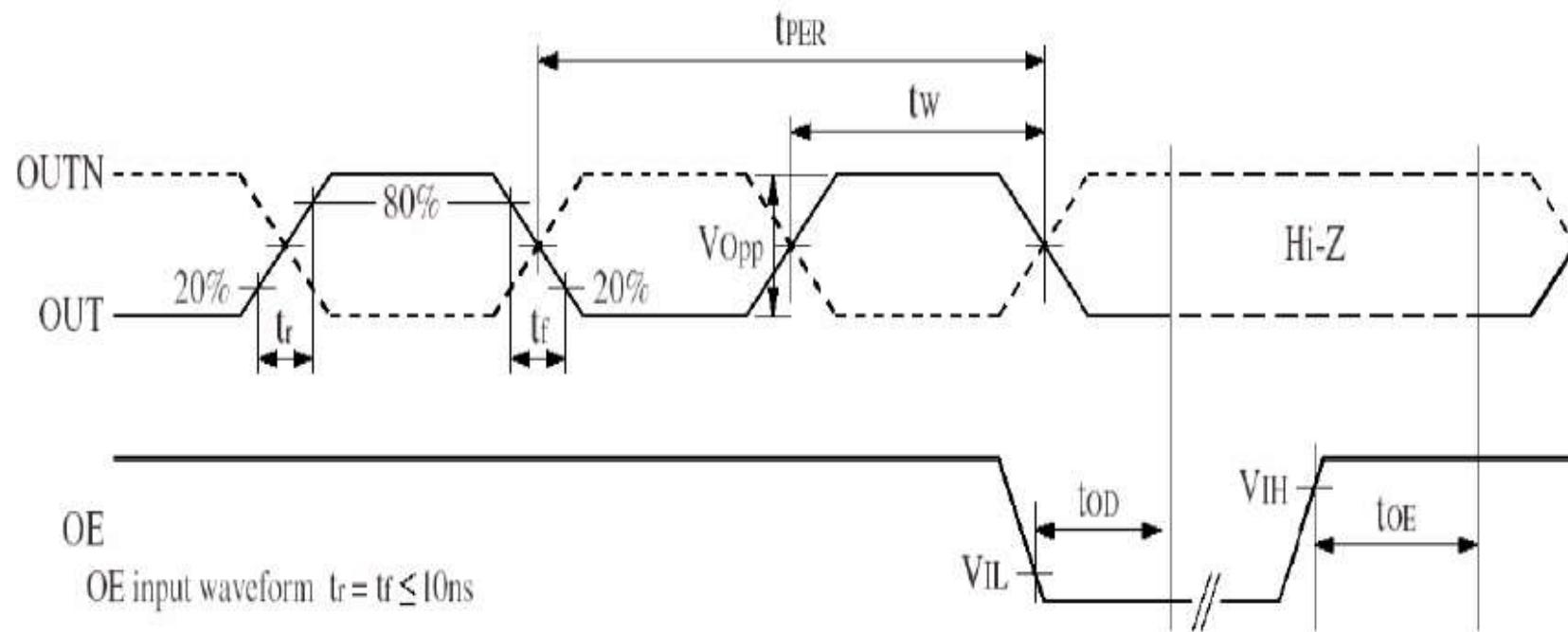
$$\begin{aligned} \text{DUTY1} &= 100t_w/t_{PER} (\%) \text{ @ crossing point} \\ \text{DUTY2} &= 100t_w/t_{PER} (\%) \text{ @ 50\% waveform} \end{aligned}$$
