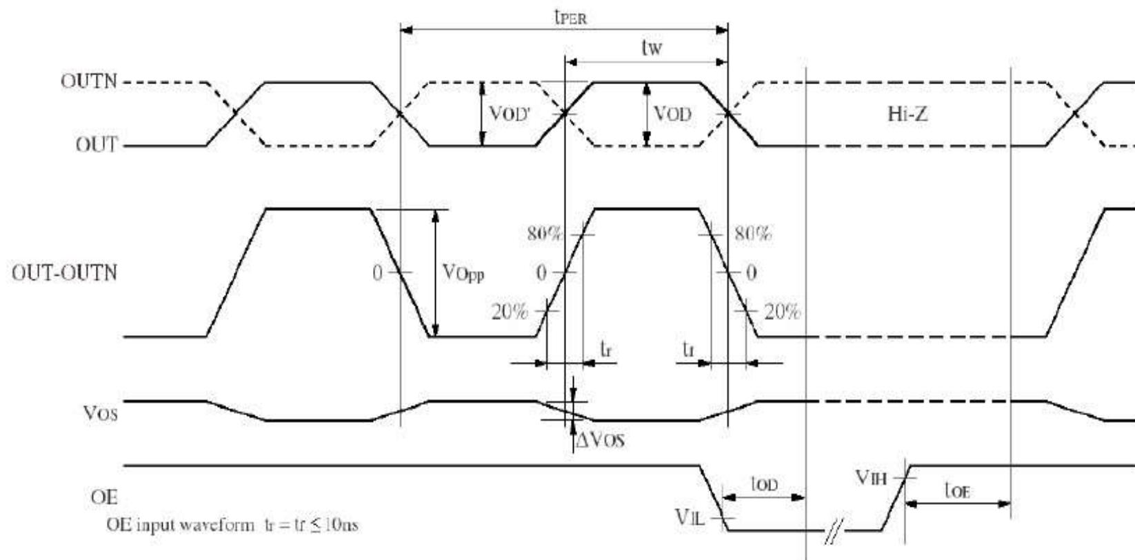
$$\text{DUTY} = 100t_w/t_{\text{PER}} (\%) \text{ @ crossing point}$$
