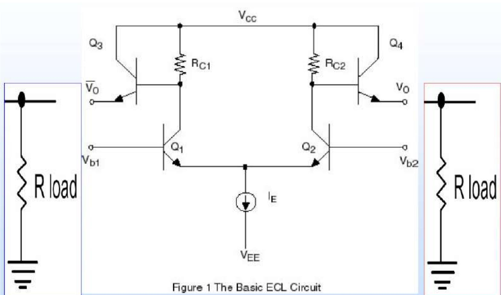
Figure 1 The Basic ECL Circuit
